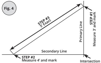
Measure three of anything: feet, yards, or any unit. Use feet-yards (meters) in big rooms. Measure 36 in. (914.4 mm or three units) on one line. Mark 48 in. (1219.2 mm or four units) on the other and measure the distance between marks. It should be 60 in. (1524.0 mm or five units) exactly. If not exactly 60 in. (1524.0 mm or five units), adjust the secondary line by pivoting on the intersection point until the diagonal reads
