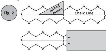
Once the left and right sides are trimmed and inserted into the first row, it's time to trim the top portion of these grids. Snap a chalk line on the back side for square and screw a board to the backside – see Figure 3.
